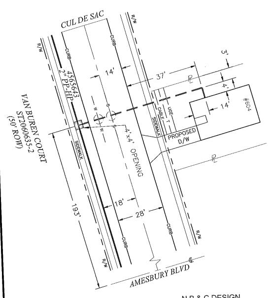
INSTALL FOOTAGE:<u>73'</u> TYPE:<u>3/4" PP</u> EFV SERIES: 1100 (\_X\_) 1800 (\_\_\_) N/A (\_\_\_) N B & C DESIGN
